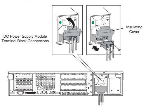
The product is supplied with an insulating cover over the terminal block. To gain access to the terminals, apply gentle pressure to flip up the cover, while using a small flat blade screwdriver to unlatch each side in turn. When the wiring is complete the cover must be flipped down, and securely latched at both sides. All wiring terminals connected to the DC power input terminal block must be insulated, with no accessible bare metal when the cover is closed.
